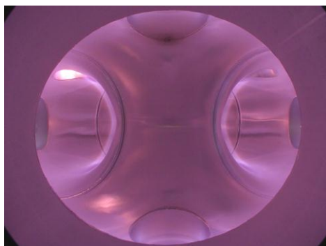
Fig 7 GDC in Argon; Helium (giving turquoise glow) is more commonly used as argon is slow to remove
