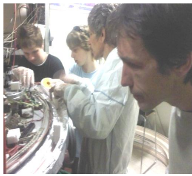
Fig 4 Commissioning the HTS poloidal field coils on the GOLEM tokamak in Prague
