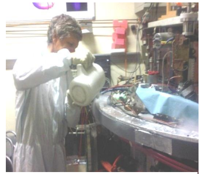
Fig 4 Commissioning the HTS poloidal field coils on the GOLEM tokamak in Prague
