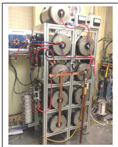
Fig 6 bank of Tavrira Supercapacitors 8 Farad in total (the top capacitor is used as a buffer for waveform control, typically to obtain flat-top).
