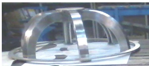
Fig 11 Upper PF coil, wound using HTS tape, undergoing cooling tests (20K using helium gas)
